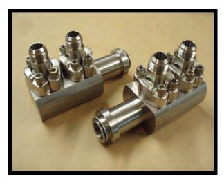
The Manifold Supply Headers are designed to be mounted on an existing valve such as a POCV, or to any existing port connector to add a secondary supply connection. Recommended hardware for mounting the manifold to the POCV is the existing hardware supplied with the POCV. The new outlet connections are 1" and/or 1-1/2" Code 62 Seal-Sub with SAE adapters used to convert to hose connections as needed.
