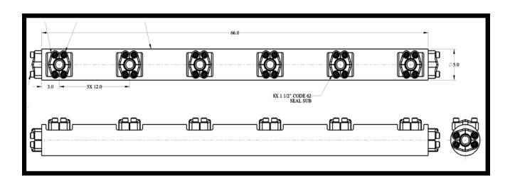
DTL can manufacture accumulator manifolds for multiple bottles with Code 62 Seal Sub, NPT, or any other connection preferred.
